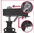
Tighten the actuator with bolts and nuts
