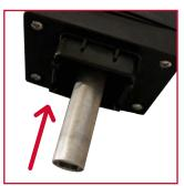
Secure the shaft to the actuator
